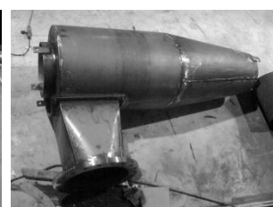
Single or multi-cyclones for de-foaming usually with significant liquid in the feed
