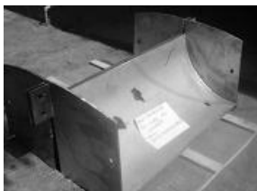
Top entry flow splitter for low-medium velocity and higher proportions of liquid content
