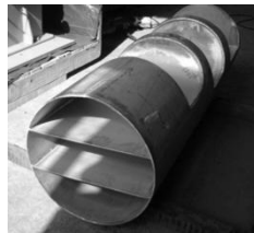
Fig. 2. Typical inlet distributors (photos courtesy HAT International Limited)
