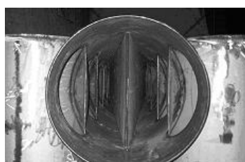
Single or multi-cyclones for de-foaming usually with significant liquid in the feed
